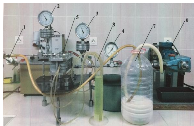
Figure 1. Laboratory equipment with a replaceable plate and frame membrane module
