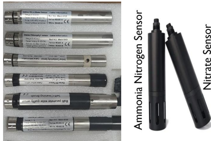
Fig. 3. Water quality monitoring sensors.
