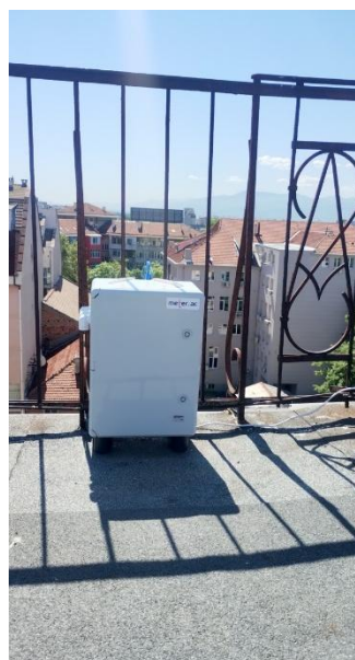
Fig. 2. View of the assembled monitoring device deployed at the rooftop of the Rectorate building, Plovdiv University (PU).
